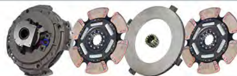
15-1/2" x 2" Easy Effort Clutch - 2-Plate - 6-Paddle - 6-Spring - Triple-Zerk with Spline Saver - 2250 Torque - 4200 Plate Load Part # ETP-EA60289TP
