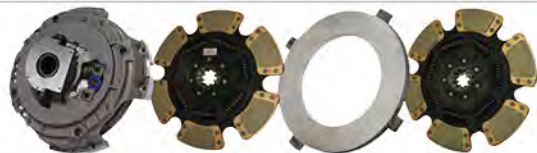
15-1/2" x 2" Easy Effort - 7-Spring - 6-Paddle - 2050 Torque - 4000 Plate Load Part# ETP-308925-25
