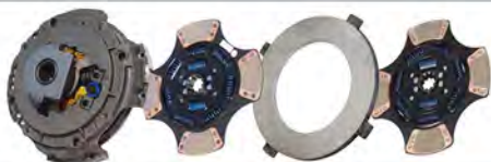
15-1/2" x 2" Easy Effort Clutch - 2-Plate, 4-Paddle - 9-Spring - Triple-Zerk - Mack - 1760 Torque - 3600 Plate Load Part# ETP-308925-51
